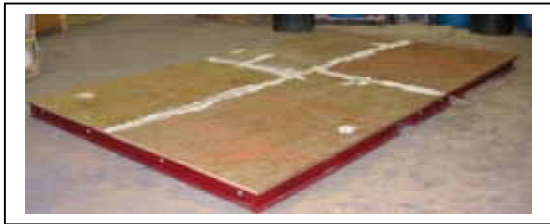
Fig. 2a ¾ Inch Plywood Decking for Floor
