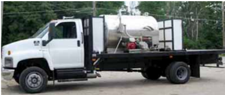
This unit can pump, power wash and replenish chemical from both sides.
