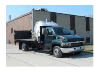
Pump Truck Lift Gate 600 Waste 250 internal Water Tank
