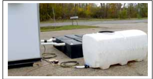
Holding Tank and Garden Hose Connection
