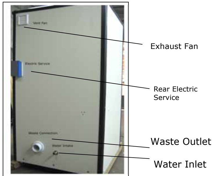
Fig. 8 Rear View Plumbing Connections
